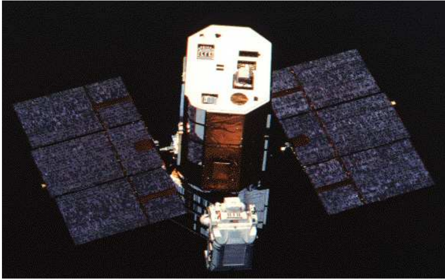
Figure 1.2: The Solar Maximum Mission (SMM) satellite was operated during 1980–1989. Some instrument failures occurred early in the mission, such as the position encoder of FCS and several gyroscopes. Repairs of the satellite were performed by “Pinky” Nelson and Dick Scobee from the Space Shuttle Challenger in April 1984. The approach of the maneuvering astronaut in his flying armchair to the ailing spacecraft is documented in this figure (courtesy of NASA).
