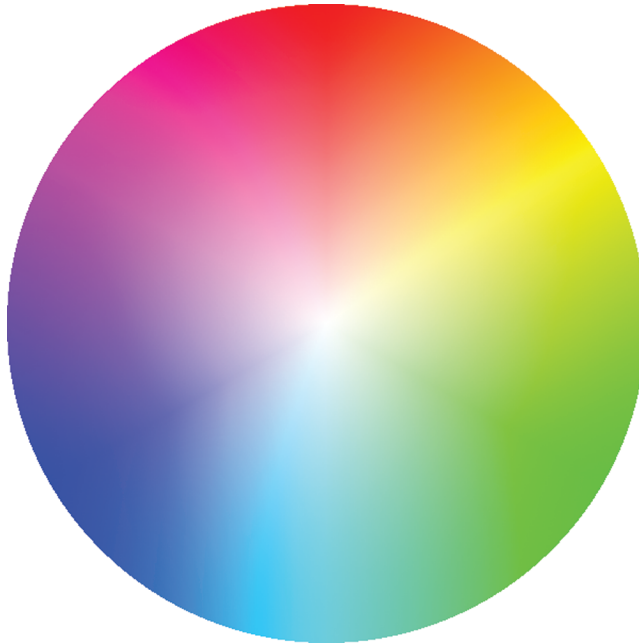
FIGURE 21.1 Example of a color wheel created using the HSV color system. In this case the value v is set to 1.0. (HSV_WHEEL_PS)
