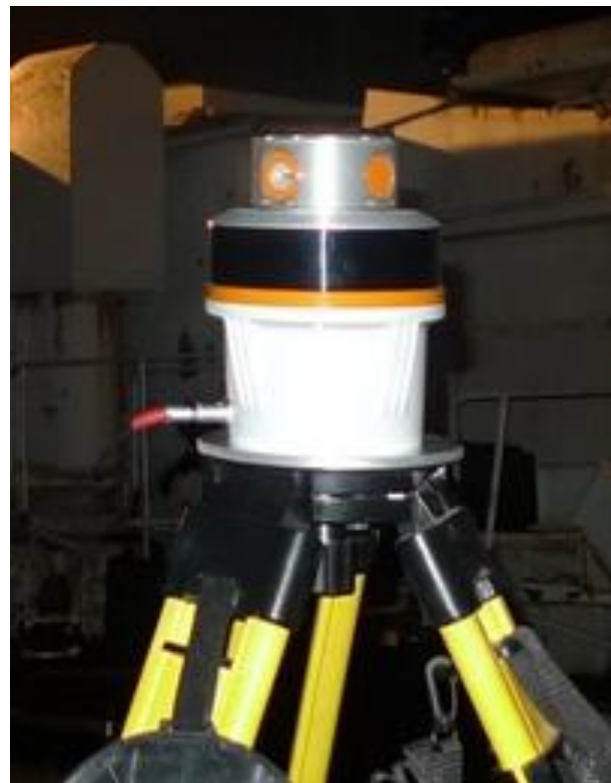
Figure 5. A transmitter of IndoorGPS
