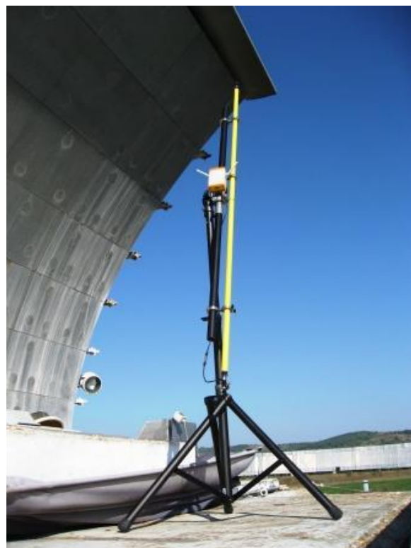
Figure 6. The two-meter calibrating rod of INDOOR GPS
